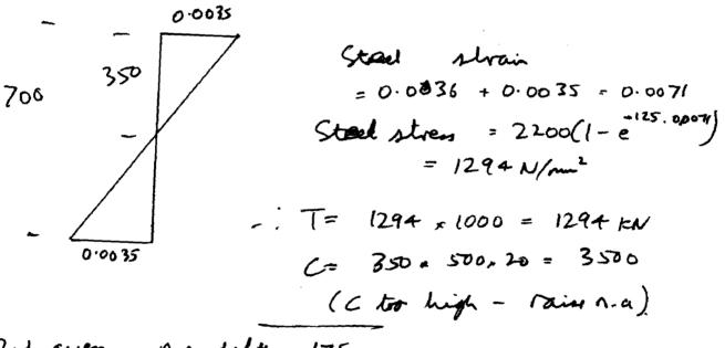
2rd guess N.a. defith = 175 mm Steel stress = 1958 N/mm<sup>2</sup> - T = 1958 KN C = 175 x 500x 20 = 1750 KN
