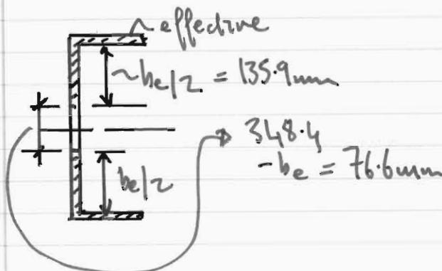
$$A_{\text{eff}} = 70.1 \text{ cm}^2 - 76.6 \times 10.4 \text{ mm}^2 \\ = \underline{\underline{6213 \text{ mm}^2}}$$
