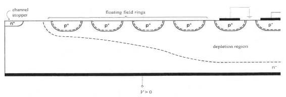
A similar result can be obtained with the junction termination extension. This is based on having regions of lowly doped p- layers spread out uniformly the electric field at the edge of the device. The p- layers have to be depleted at breakdown.
