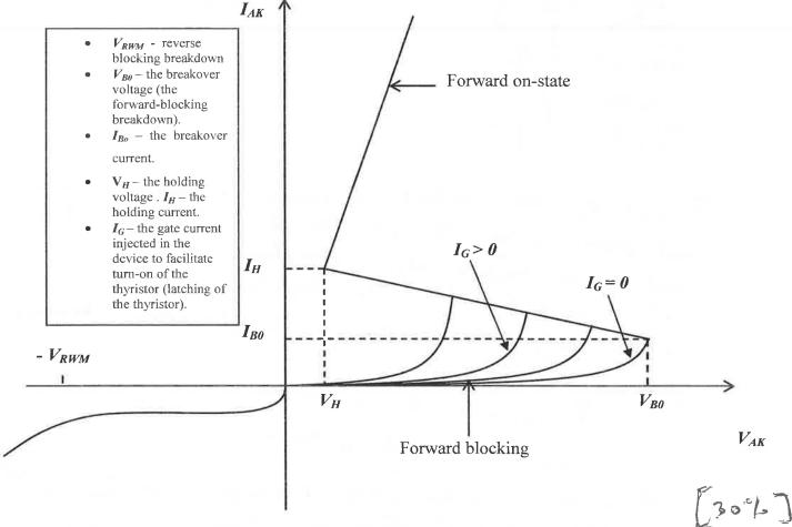
(b) This effect is very severe during turn-off when a high forward voltage is re-applied to the structure. There is a maximum dV/dt rating above which the displacement current created through the junction capacitance will be greater than the breakover current, thus resulting in a parasitic re-turn-on (the device refuses to turn-off).
