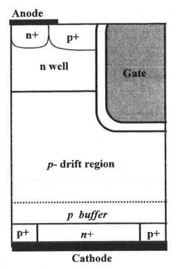
The p+ shorts are connected together with the n+ electron emitter to the cathode terminal. The device could be used in the high side with the anode as high voltage terminal. It features a p-channel and p-drift region. When the gate is negative with respect to the anode and the inversion layer is formed, holes can travel from the p+ anode through the channel to the p-drift region and are collected by the p+ shorts. Once the n+/p buffer junction becomes
