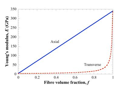
The inverse rule of mixtures gives the accompanying graph for transverse stiffness, the axial stiffness is linear with fibre content.
