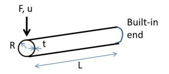
(b) The end deflection is  $u = \frac{FL^3}{3E_1I}$  where  $I = \pi R^3 t_0$ For CFRP, this gives  $t_0 = \frac{FL^3}{3\pi E_1 R^3 u} = \frac{1 \times 10^3 \cdot 3^3 \times 10^3}{3 \cdot \pi \cdot 138 \times 10^3 \cdot 20^3 \cdot 0.5} = 5.18$  mm, and a total wall thickness
