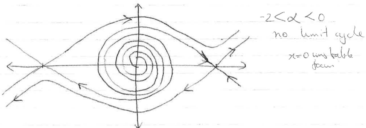
(d) Hopf bifurcation. Transition from stable focus to unstable focus with the system describing transition from decaying oscillation to unstable growth with an intermediate region showing stable limit cycle oscillation (NOTE  $z^3$  term).
