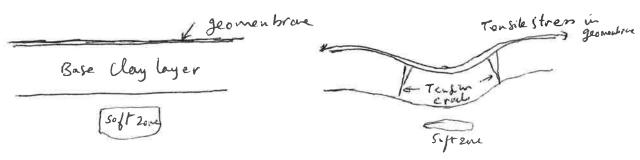
If peat zones are detected before the base layer is placed, use of geo-grids to locally stuffen the sail is recommended. These geo-grid are both effective solution if the lateral extent of the soft zone is limited.
