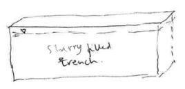
Soil-bentonite stury is introduced into the trench, and excavation is continued below the Slurry. The Soil-bentonite surry provides the lateral stability to the trench. It is very important to maintain the
