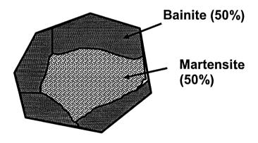
For the  $\frac{1}{2}$  NiCrMo steel: Air cool:  $D_0 = 1$  mm Oil quench:  $D_0 = 22$  mm Water quench:  $D_0 = 32$  mm
