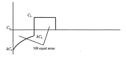
Move molten zone of width L a distance  $\delta L$  from x to  $x + \delta x$ , area A.
