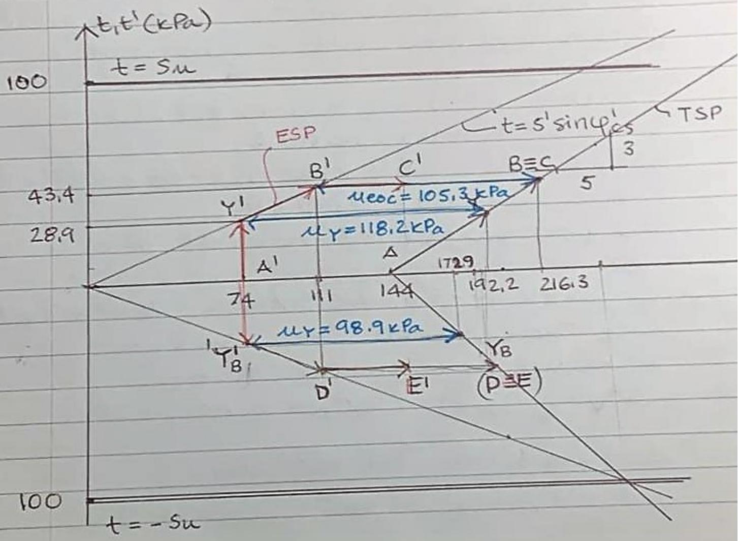
(c) Before embankment construction, the stress state at point B is the same as at soil element A.
