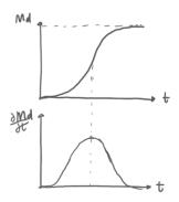
Md: total mass of drug release; dMd/dt: rate of drug release. Assumptions: the hydrolysable polymer is used as the carrier for cancer drugs, where the drugs are homogenously dispersed into the matrix. The polymer undergoes matrix erosion resulting in drug release, and the rate of drug release is directly related to the rate of matrix erosion due to hydrolysis.
